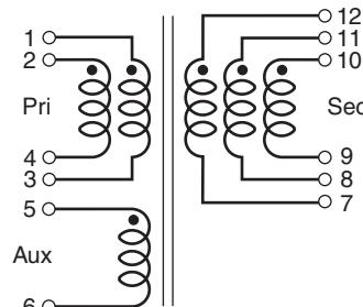
The primary windings and the secondary windings to be connected in parallel on the PC board.
